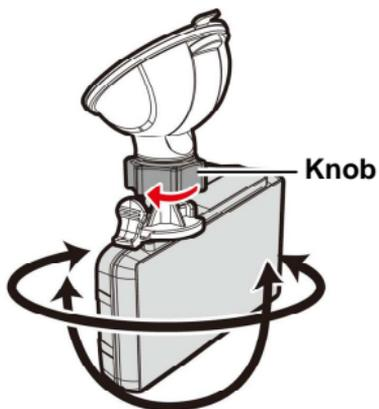
2. Then tighten the knob to make sure the device is securely locked in place.
