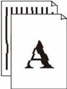
Lines Are Misaligned/Distorted
