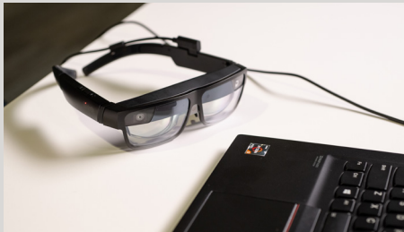
Tethered-attach AR to Windows PC
