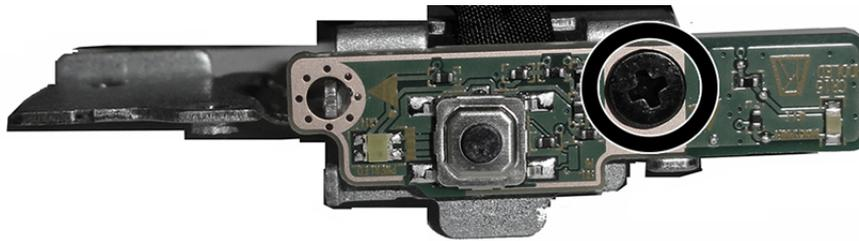
To install the power button and fingerprint sensor boards, reverse the removal procedures.
