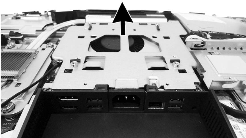
8. If it is necessary to remove the fan from the bracket, remove the four Torx screws that secure the fan to the bracket.
