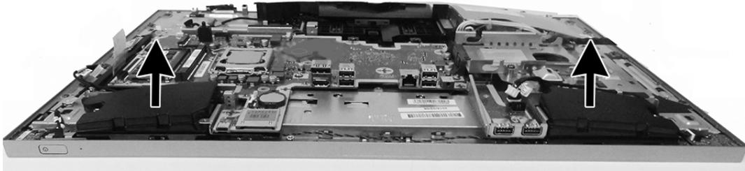
To install the speakers, reverse the removal procedures.
