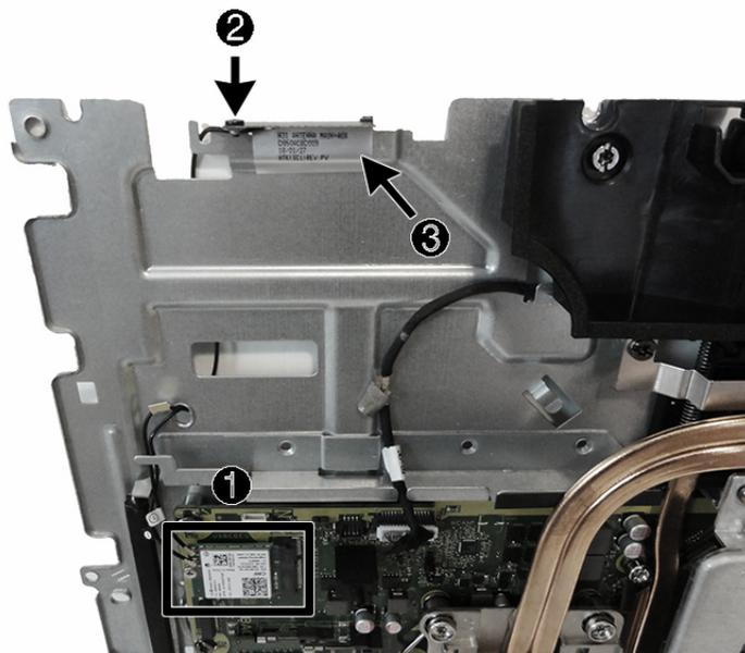
12. Remove the Phillips screw from the left antenna (1), and then peel the antenna from the chassis (2).
