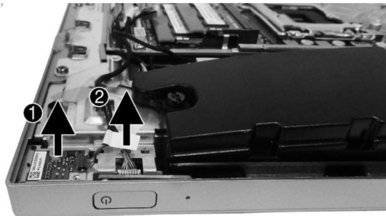
7. If necessary, disconnect the cables from each board.
