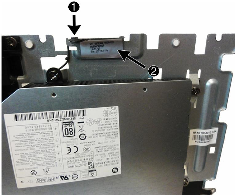
13. From the back of the frame, pull the antenna cables through the hole in the frame (1).
