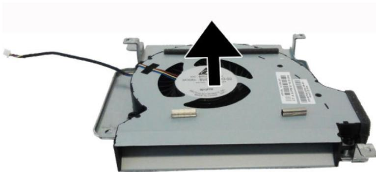
To replace the VESA mounting bracket/fan assembly, reverse the removal procedures.
