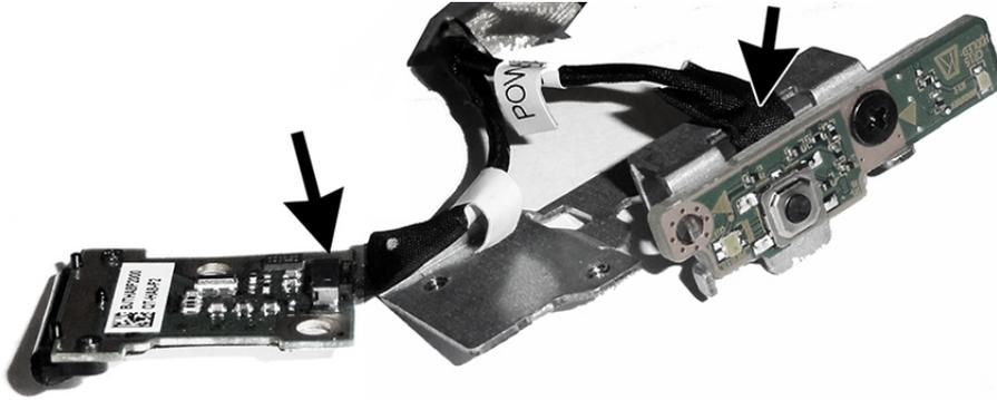
8. If necessary, remove the Phillips screw that secures the power button board to the bracket, and then remove the board from the bracket.
