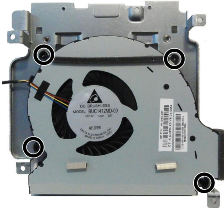
9. Separate the fan from the bracket.
