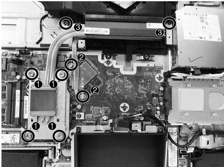
9. Lift the heat sink out of the computer.
