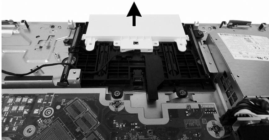
12. If you need to remove the webcam bracket, remove the VESA bracket/fan assembly ([VESA mounting bracket/fan assembly on page 48](#)), and then remove the four Torx screws (1) that secure the webcam bracket to the computer.
