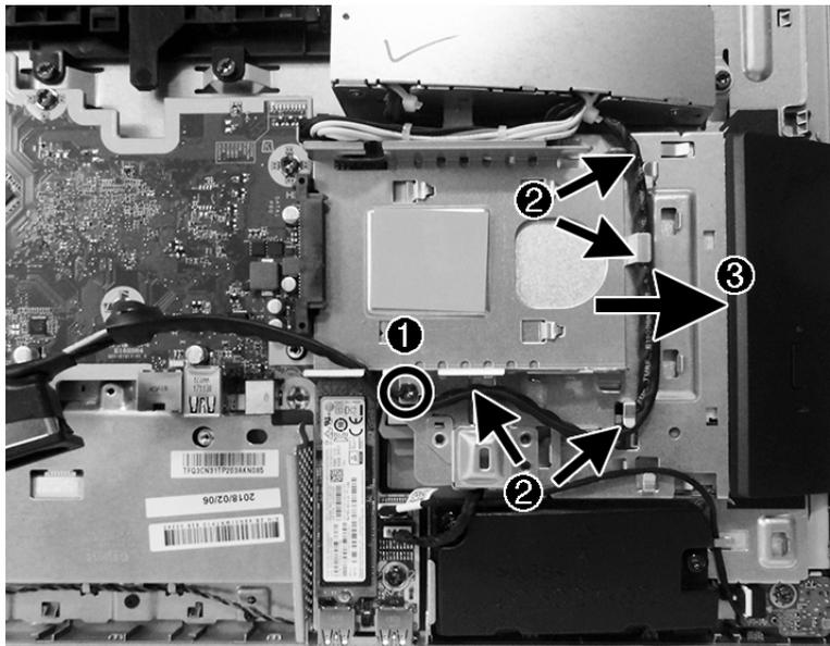
To replace the hard drive cage, reverse the removal procedures.
