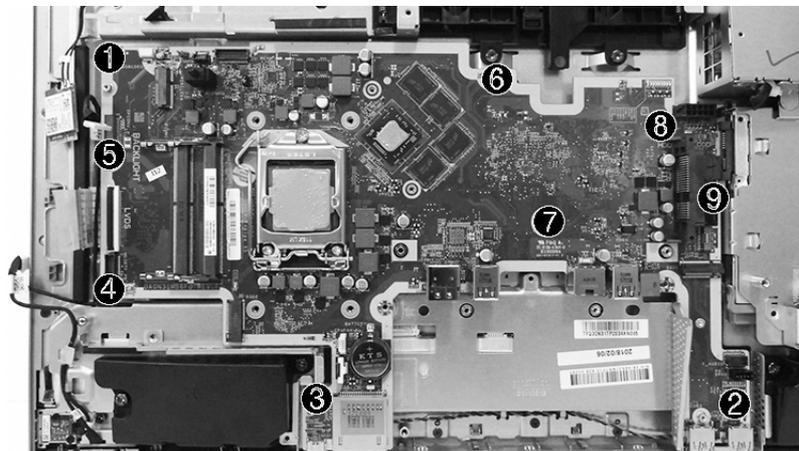
**16.** Lift the system board up and out of the computer.
