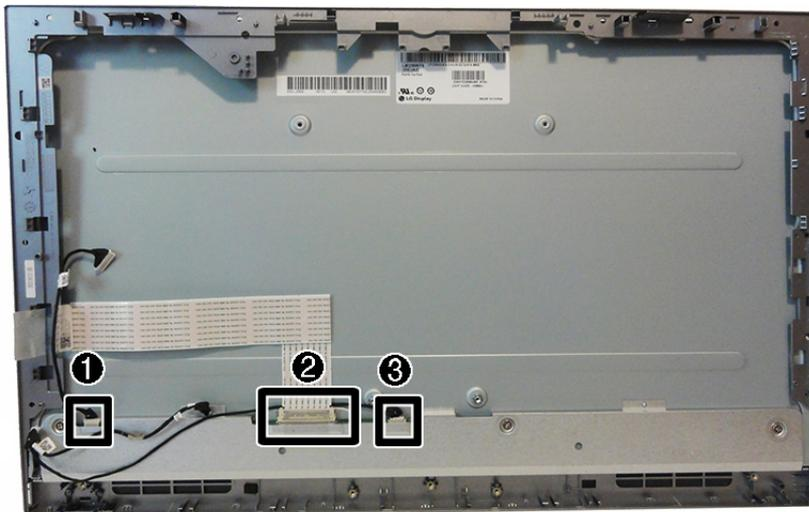
17. Separate the middle frame from the display by sliding the bezel down, and then removing it from the display.
