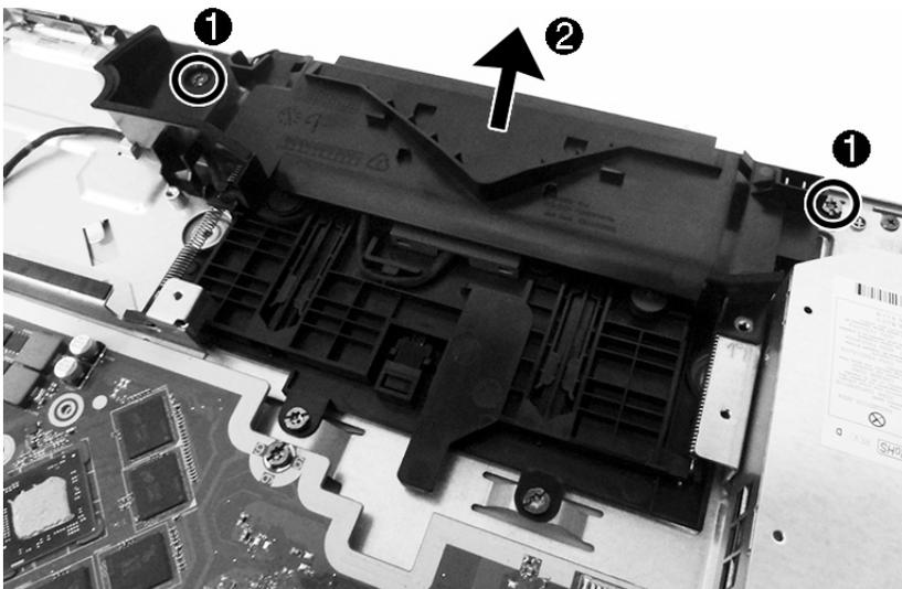
8. Remove the two Phillips screws **(1)** that secure the webcam assembly to the computer.
