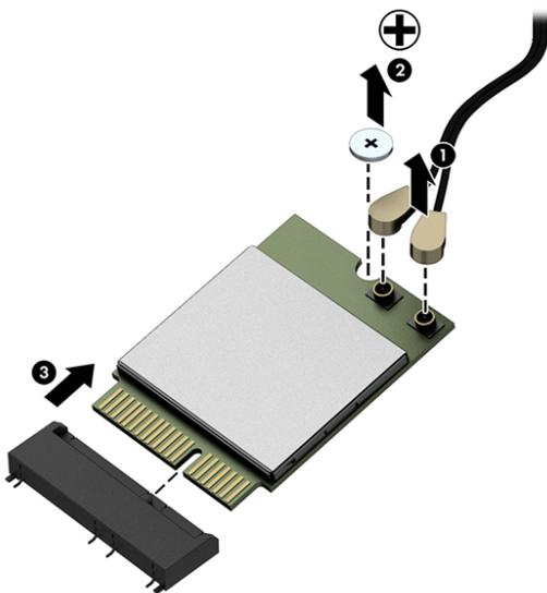
To install the WLAN module, reverse the removal procedures.
