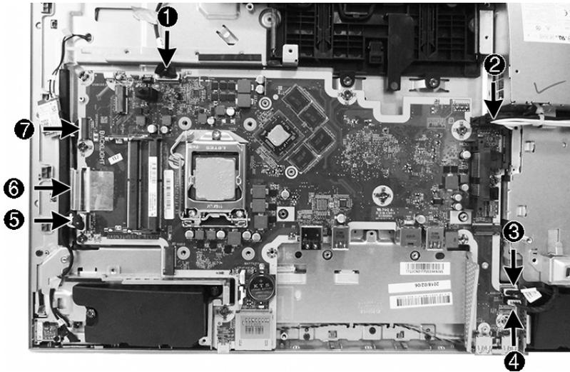
**15.** In the order printed on the system board, remove the nine Torx screws **(1)-(9)** that secure the system board to the computer.
