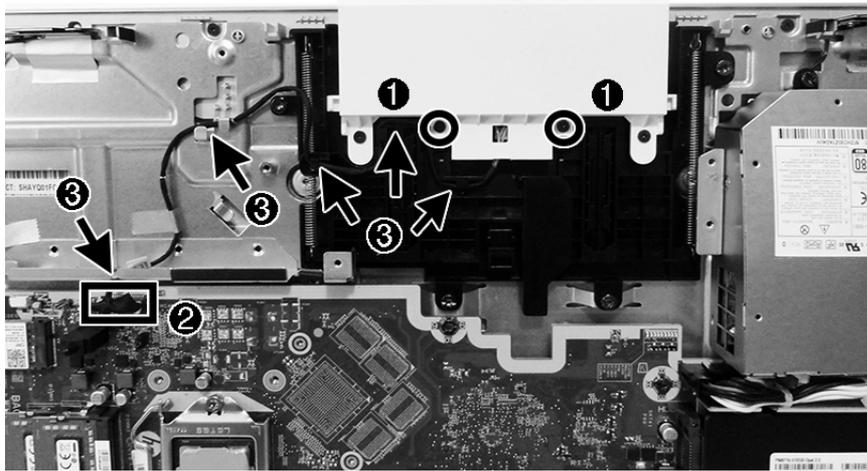
11. Remove the webcam assembly from the computer.
