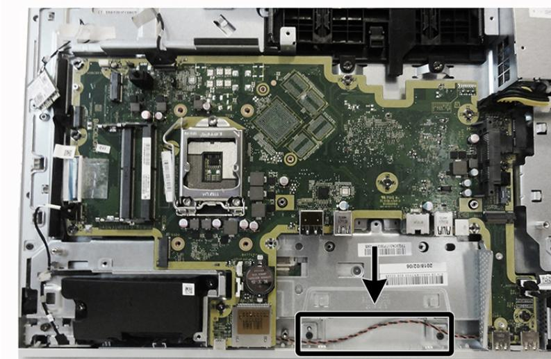
To remove the RFID board:
