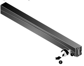
**Step 3** Hook the front bezel onto the side of the left mounting ear, and press the button so that the front bezel is secured to the chassis. See **Figure 5-5**.
