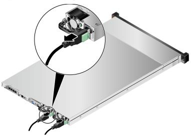
**Step 4** Press the spring on the PSU in the arrow direction, and pull the PSU out of the slot while holding the handle. See steps (1) and (2) in **Figure 5-13**.
