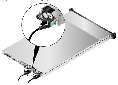
**Step 4** Secure the power cable using a cable tie. See **Figure 5-18**.
