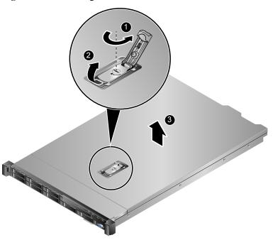
Figure 5-22 Removing a chassis cover
