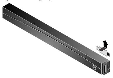
**Step 2** Unlock the front bezel by turning the key clockwise, and remove the key for proper storage. See **Figure 5-4**.
