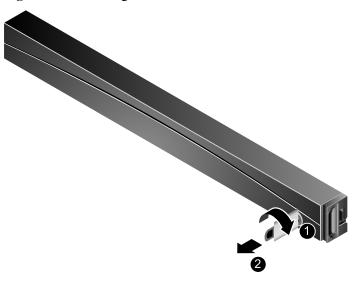
**Step 2** Press the button and remove the front bezel. See Figure 5-2.
