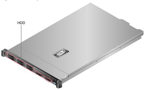
**Step 3** Fully raise the ejector lever and push the hard disk into the chassis along the guide rails until it does not move. See step (1) in **Figure 5-10**.
