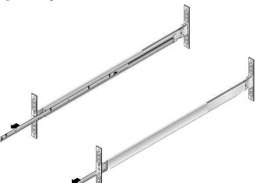
Figure 2-8 Pulling out inner rails
