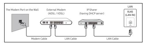
• Depending on how your network is configured, you may be able to attach your product to your LAN by connecting the LAN port on the back of your product directly to a network wall outlet using a LAN cable.
