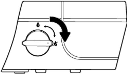
After moving the product and before you print, make sure the ink valve is unlocked, allowing the printer to function properly. Turn the valve completely to the left (vertical position) to unlock.
