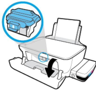
6. Push down to open the blue printhead latch.
