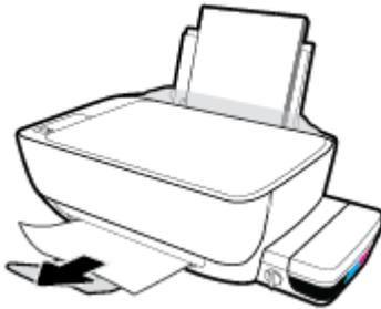
3. Press the **Resume** button (
