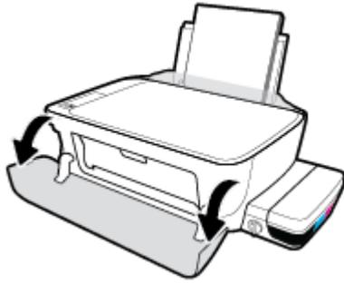
5. Open the printhead access door and wait for the print carriage to move to the center of the printer.
