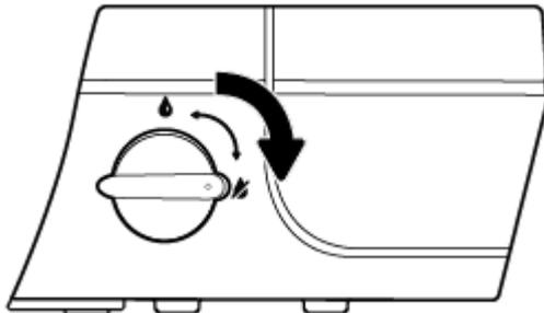
After finishing clearing the paper jam, turn the ink valve to the unlocked position.
