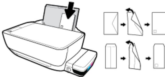
4. Slide the paper-width guide to the right against the stack of envelopes until it stops.
