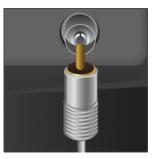
Oconnect the CATV cable or TV antenna cable to the "ANT IN" port on the rear side of the product. Make sure to use a TV antenna cable (sold separately) as the antenna cable.
