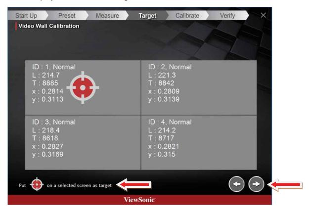
m. Mouse over to display to be calibrated and place the color pod over the "white" area of the gear. Click on the box. The calibration process for that display will begin. Wait for it to complete.
