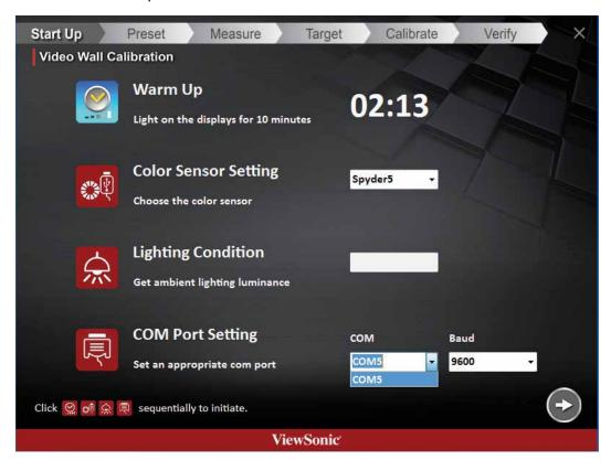
c. When the timer reaches 00:00, then click on the Color Sensor Setting button. Place the Spyder5 pod on the central area of the video wall and click Lighting Condition to get the ambient light reading. Click on the COM Port setting button to lock it in. Then click on the right arrow to move to the next step.
