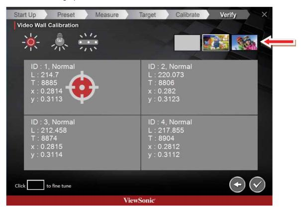
q. This is the fine tuning dialogue box. You can click measure to get the current reading of a specific display.
