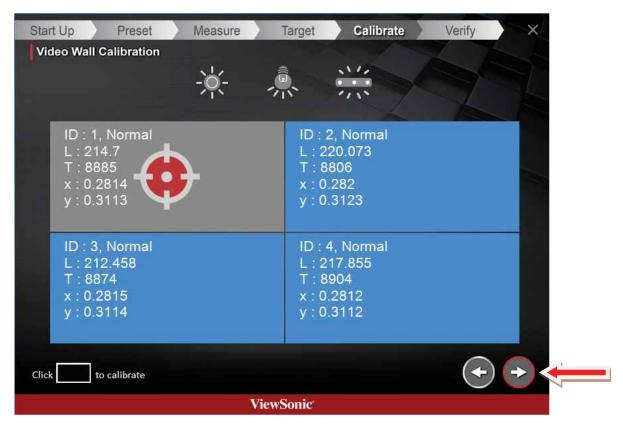
p. This is the verification stage. You can select each image to visually compare the images. You may mouse over any display and place the pod over the "white" area of the gear if you want to fine tune a specific display. Click on the box to bring up the fine tune screen.
