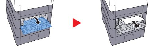
**NOTE** If the paper cannot be removed, do not try to forcefully remove it.
