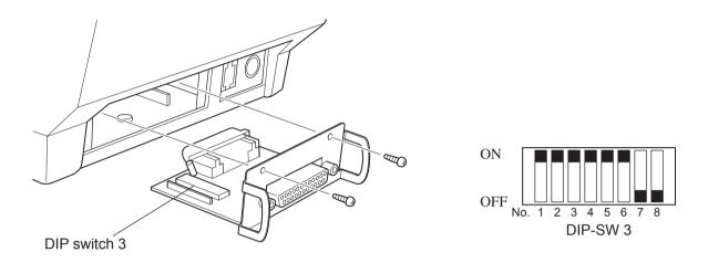
The factory settings of DIP switch are all on, except for switches 7 and 8.
