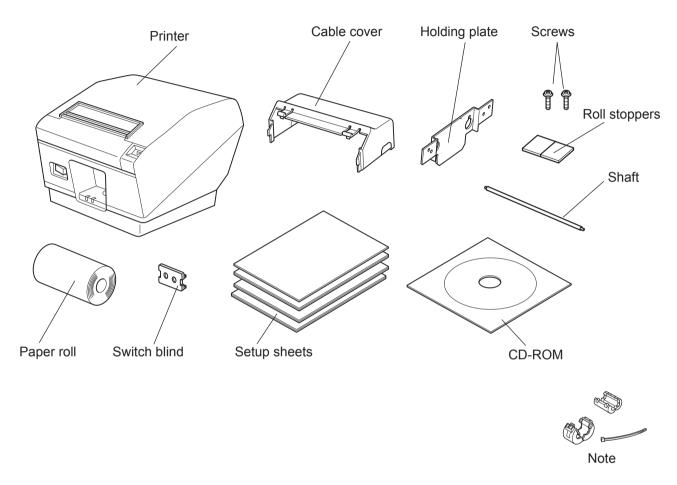
**Note:** The ferrite core and fastener provided with your printer depend on your printer configuration.
