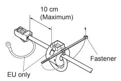
③ Loop the fastener around the cable, and then pull the end of the fastener tightly through its buckle. Use a pair of scissors to cut off the excess end of the fastener.
