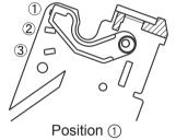
Paper thickness between 65 μm and 105 μm
