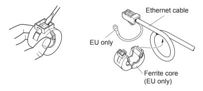
2 Pass the fastener through the holes in the ferrite core as shown in the illustration.
