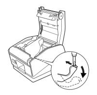
As shown, use a flat head screwdriver to move the adjustment lever inward. Then, lower the adjustment lever to the position in which the protrusion on the adjustment lever engages with the hole in the frame.
