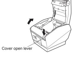
Set the paper roll in the direction as shown, and pull on the leading edge of the paper towards you.
