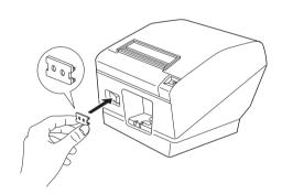
The power switch can be turned ON (  $\rm I$  ) and OFF (O) by inserting a narrow instrument (ball penetc.) in the holes in the switch blind.
