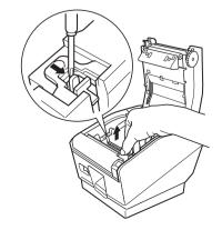
(4) Attach the holding plate to the printer. Then tighten the two screws that were supplied to secure it in place.
