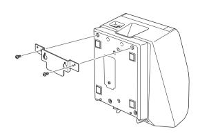
(5) Position the printer over the screws, etc., on the wall and then slide it downward to set it in place.
