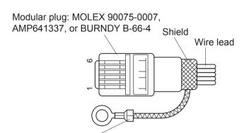
Separated Ground wire connected to shield (Europe only).
