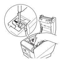
Use a flat head screwdriver as shown to remove the clips at both ends of the tension bar. Then, remove the tension bar unit.
