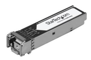
The SFPGE10KT5R3 is a Juniper SFPP-10GE-LR compatible fiber transceiver module that has been designed, programmed and tested to work with Juniper brand switches and routers. It delivers dependable 1 GbE connectivity over fiber cable, for 1000Base-BX10-D compliant networks, with a maximum distance of up to 40 km (24.8 mi).
