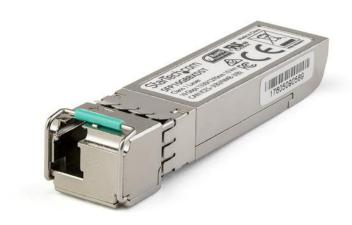
The SFP10GBX10DS is a Dell EMC SFP-10G-BX10-D compatible downstream fiber SFP transceiver which pairs with StarTech.com's SFP10GBX10US. They are designed, programmed and tested to work with 10GBase-BX10 compatible Dell EMC switches and routers. The SFP+ transceiver module supports a maximum distance of up to 10 km (6.2 mi) and delivers dependable 10 GbE connectivity over fiber cabling.
