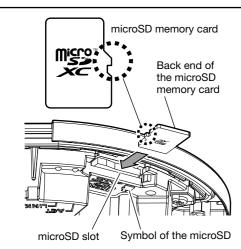
• Back end of the microSD memory card does not protrude over the surface line of the microSD slot.
