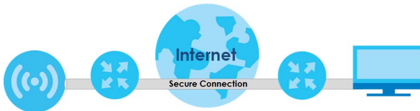
Figure 95 SSH Communication Over the WAN Example
