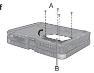
4 Insert/Remove the RAM module.
