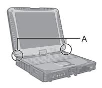
Use the tether to attach the stylus to the computer so you will not lose it. There are holes (A) to attach it.
