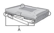
Attach the hand strap to any two of the corners (A) using the screws. You can connect the shoulder strap (B) to the hand strap. (The illustration is an example.)
