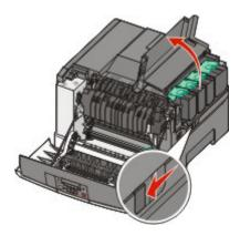
Remove the toner cartridges by lifting the handles, and then gently pulling away from the imaging kit.
