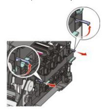
7 Press down on the blue levers, grasp the green handles on the sides, and then pull the imaging kit out.
