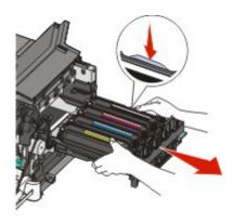
**8** Remove the used developer unit.
