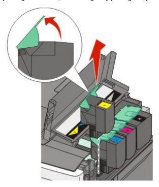
Align the new toner cartridge, and then press down until it is all the way into the slot.
