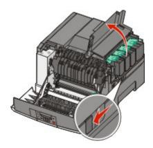
Remove the toner cartridges by lifting the handles and then gently pulling away from the imaging kit.
