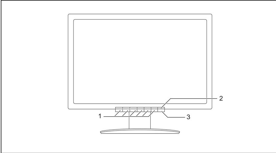
1 = Buttons for the OSD menu (On-Screen Display)      3 = ON/OFF switch
