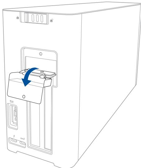
6. Remove the screws that secures the metal bracket to the XG Station PRO, then remove the metal bracket.
