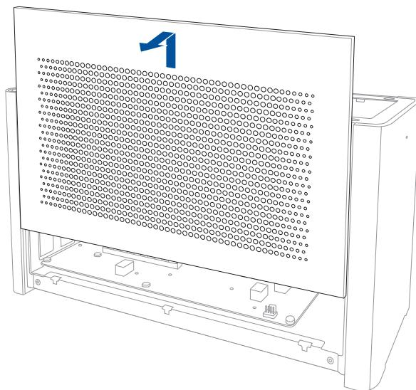
4. Remove the screw that secures the metal cover to the XG Station PRO.
