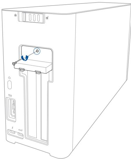
5. Open the metal cover downwards to an opened position.
