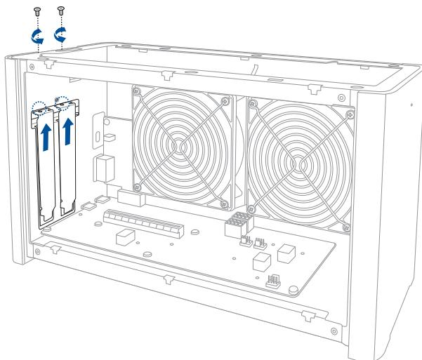
7. Align and insert the graphics card into the PCI-E slot.
