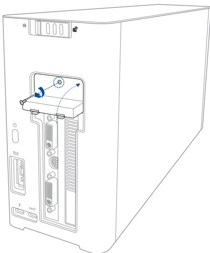
10. Align and slide the side cover into the XG Station PRO.
