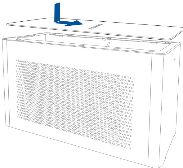
4. Slide the cover lock to the locked position.
