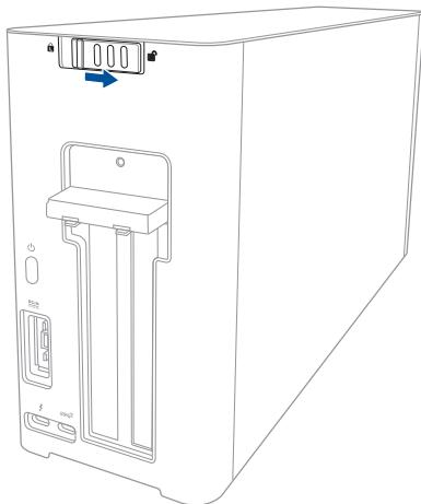
2. Slide the top cover towards the rear of the XG Station PRO, then lift the top cover open.
