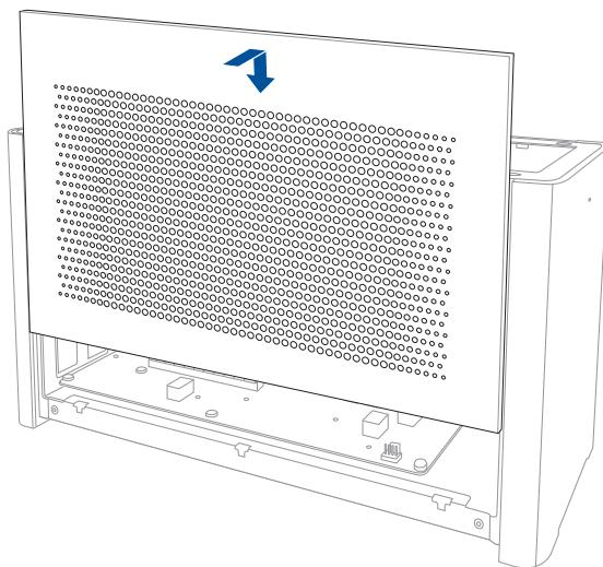
3. Align and slide the top cover towards the front of the XG Station PRO to secure it in place.
