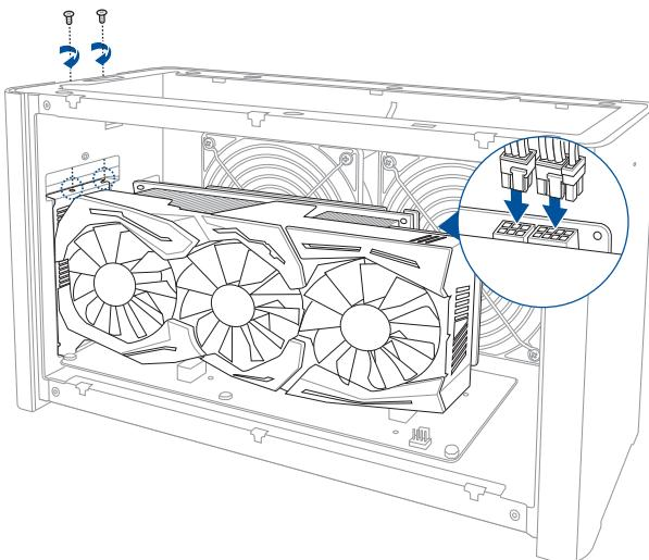
9. Lift the metal cover upwards to a closed position, then secure the metal cover with the screw that you removed earlier.
