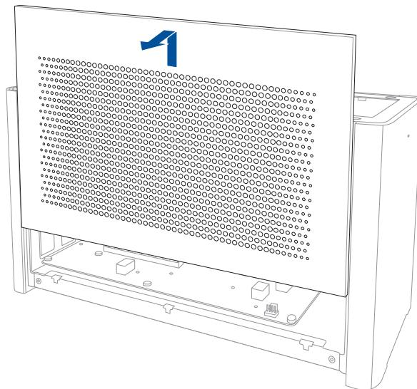
4. Slightly lift the air filter handle (A), then slide the air filter and lift it out of the side cover (B).
