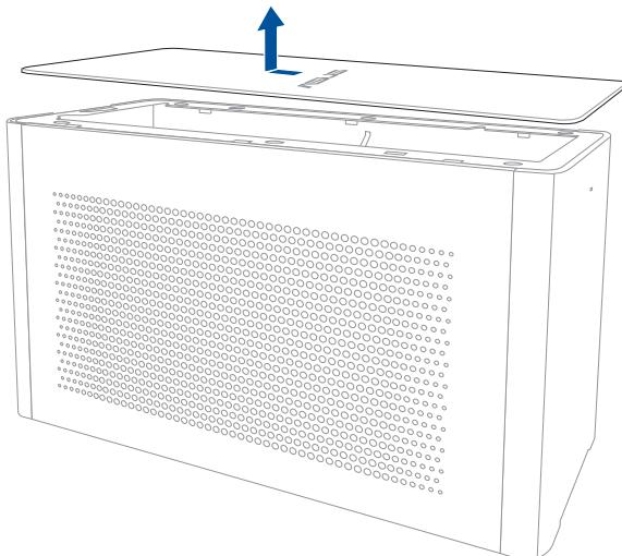
3. Slide the side cover upwards to remove it from the XG Station PRO.
