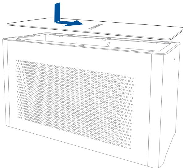
12. Slide the cover lock to the locked position.
