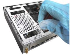
Step 5. Remove the HDD holder carefully and set it aside for later use.
