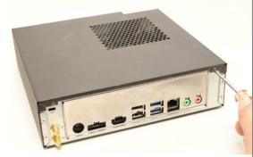
Step 3. Remove the cover carefully and set it aside for later use.
