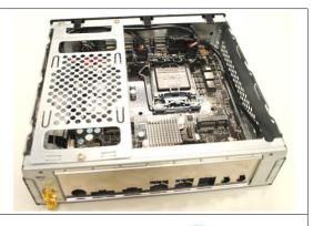
Step 4. Unlock the three screws on the HDD holder and keep them for later use.
