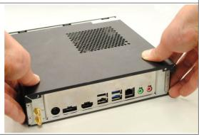
Then you can see the internal of the system. For installing CPU/ Memory module/ WIFI module/ M-SATA module, you also need to remove the HDD holder
