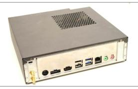
Step 2. Unlock the two screws on the back side and keep them for later use.
