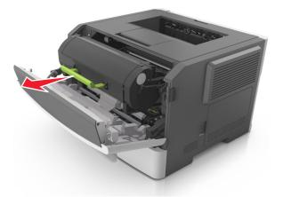
**3** Lift the green handle, and then pull the imaging unit out of the printer.
