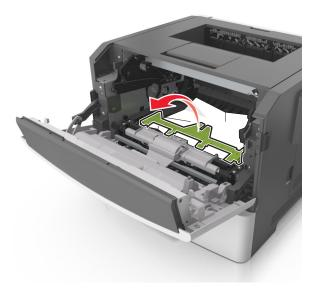
6 Firmly grasp the jammed paper on each side, and then gently pull it out.Note: Make sure all paper fragments are removed.
