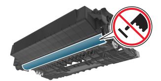
**6** Insert the imaging unit into the printer by aligning the arrows on the side rails of the imaging unit with the arrows on the side rails inside the printer.
