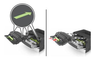
8 Insert the toner cartridge by aligning the side rails of the cartridge with the arrows on the side rails inside the printer, and then insert the cartridge into the printer.
