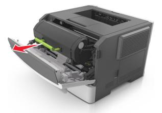
**3** Lift the green handle, and then pull out the imaging unit from the printer.
