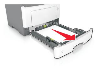
2 Firmly grasp the jammed paper on each side, and then gently pull it out.Note: Make sure all paper fragments are removed.
