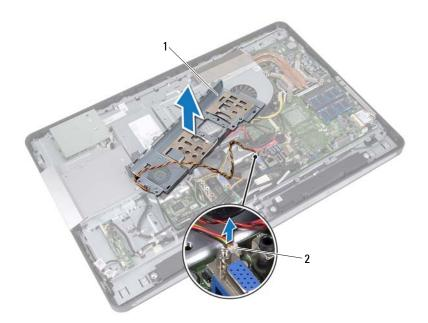
1 I/O board shield 2 power-supply fan cable
