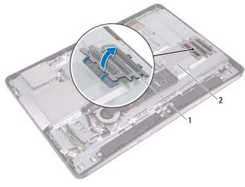
memory-module shield system-board shield 1 2
