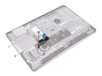
1 screw 2 power-supply fan bracket
