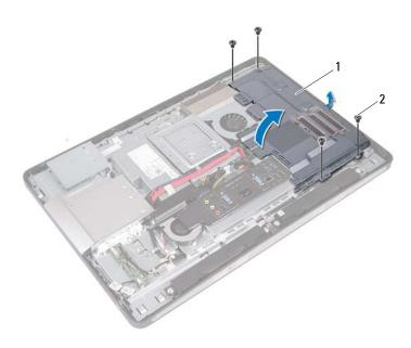
1 system-board shield 2 screws (4)
