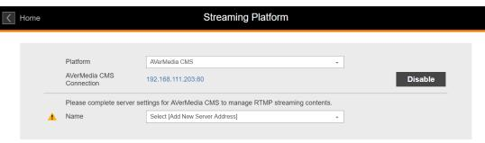
Enter an easy-to-remember name, RTMP URL and stream name. The playback URL is for the video preview function and will vary with the settings of the your RTMP server. In this case, Nginx server is providing transcoding service from RTMP to HLS.
