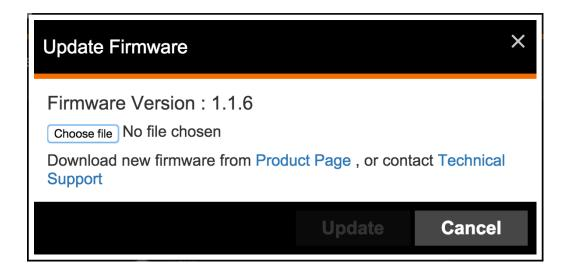
After BIN file is uploaded and verified of its integrity, confirm this dialog to proceed on the update. **DO NOT remove the power or network cable until you are prompted that the process has completed successfully.**
