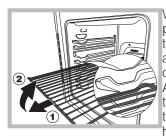
WARNING! The oven is provided with a stop system to extract the racks and prevent them from coming out of the oven.(1) As shown in the drawing, to extract them completely, simply lift the racks, holding them on the front part, and pull (2).
