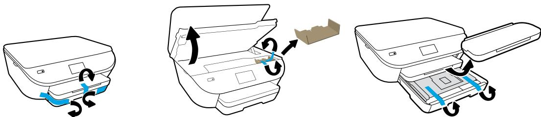
Remove tape and packing material.
