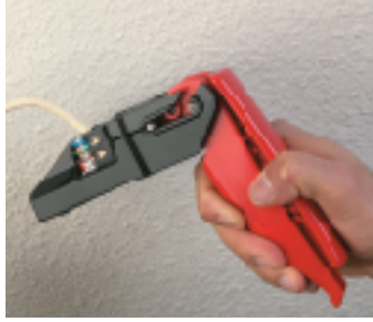
5. Pull trigger completely until you hear an audible "click".
