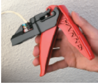
4. Ensure jack is completely and securely inserted in jack holder bed with IDC slots facing the blades.
