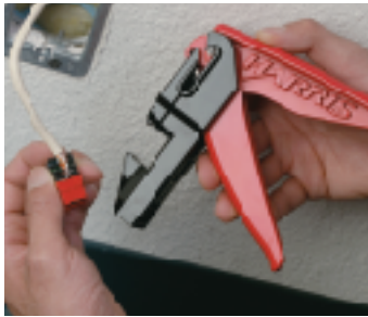
7. Release handle and remove jack from JackRapid tool. Visually verify proper termination.
