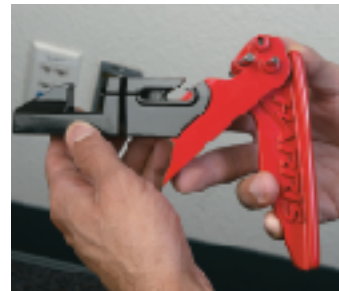
3. You have successfully removed the blade head.
