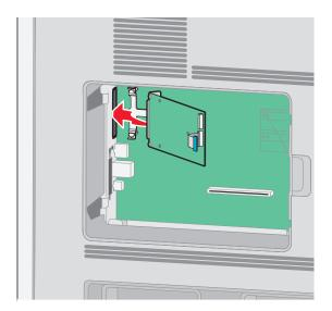
7 Lower the ISP toward the plastic tee until the ISP is seated between the guides of the plastic tee.
