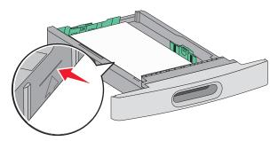
**6** If necessary, adjust the paper guides to lightly touch the sides of the stack, and lock the length guide for the paper sizes indicated on the tray.
