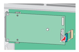
If a printer hard disk was previously installed, then attach the printer hard disk to the ISP. For more information, see "Installing a printer hard disk" on page 30.
