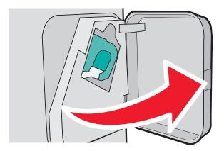
Pull the latch of the staple cartridge holder down, and then pull the holder out of the printer.
