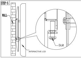
Install the bracket to the rear of the display.
