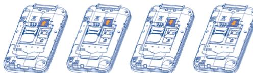
Place the microSD card with the chip facing downwards and slide it into its housing. Make sure that it is correctly inserted. To remove the card, press and slide it out.
