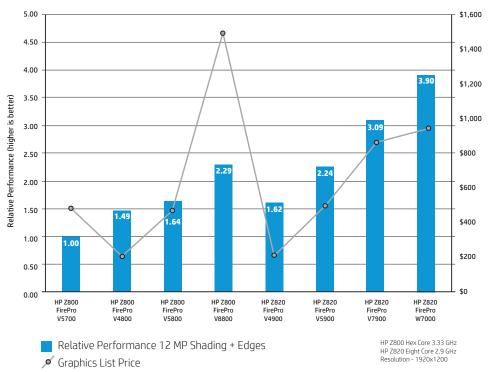
CATIA® V5R20 SP2 —CATGTSPerformance Benchmark tests VB0 graphics operations. MP = Millions of Polygons Good scaling is obtained with large models or assemblies containing large parts.
