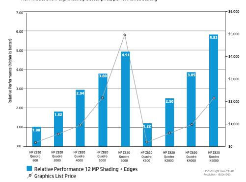
CATIA® V5R20 SP2 —CATGTSPerformance Benchmark tests VB0 graphics operations. MP = Millions of Polygons Good scaling is obtained with large models or assemblies containing large parts.
