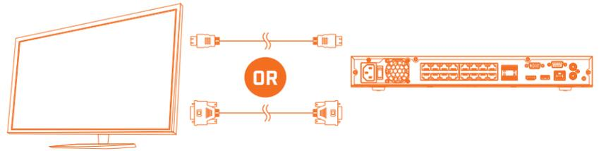
**IMPORTANT:** To optimize picture quality, set the recorder's video output to match the resolution of your monitor. See the section **Changing the Recorder's Output Resolution** on the rear for details.
