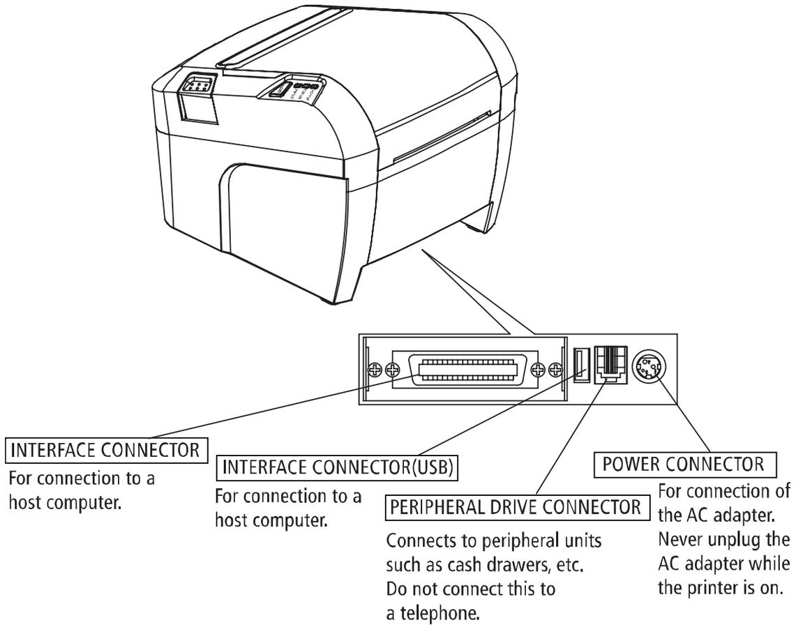
Before connecting any of the cables, make sure that both the printer and the computer are turned off.
