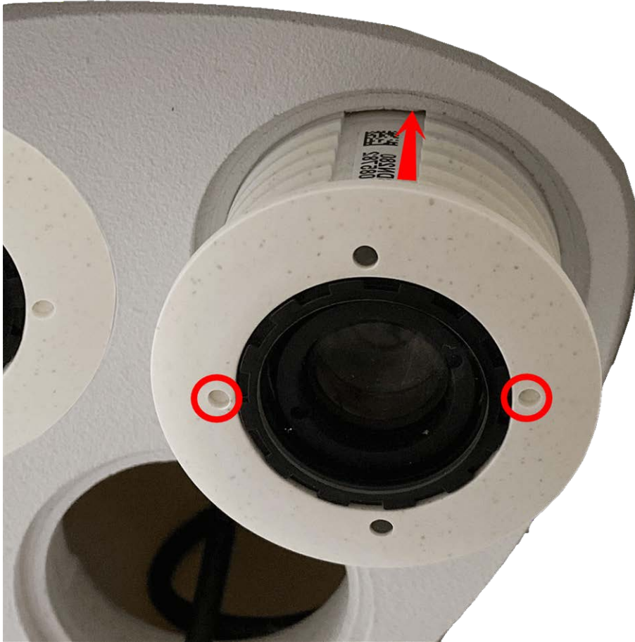
Fig. 25: Insert sensor module into Thermal front plate
