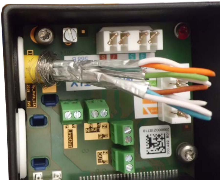
Fig. 60: Network cable inserted, plug properly seated
