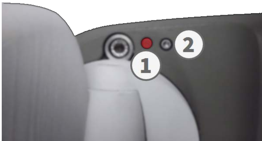
Fig. 74: View of the M73 from below with LED (1) and screw with sealing (2) that hides the key inside the camera body
