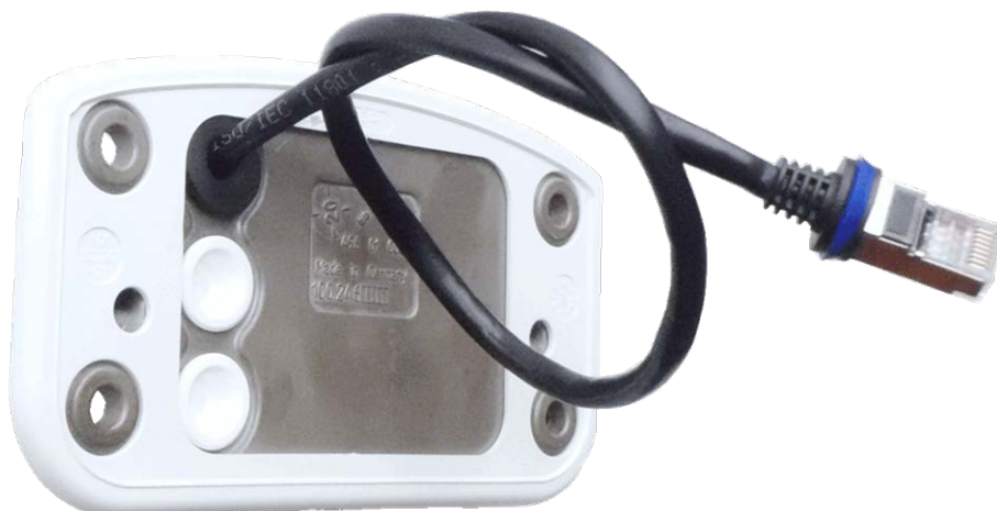
Fig. 32: Network connection of the M73
