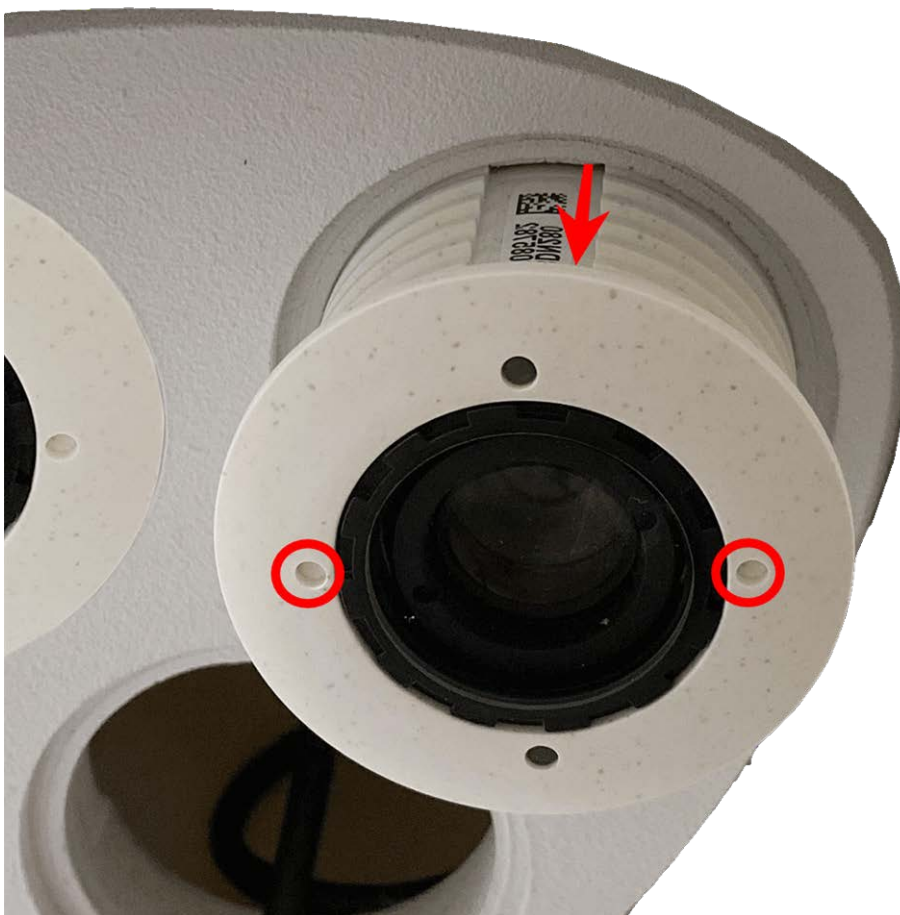
Fig. 23: Remove sensor module from the module housing
