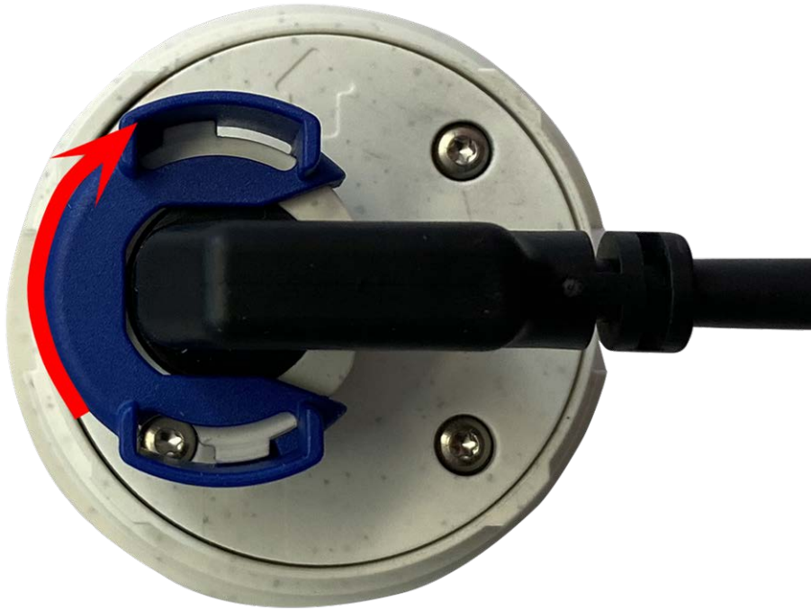
Fig. 11: Lock sensor module
