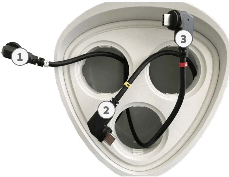
Fig. 8: Numbered sensor module cables
