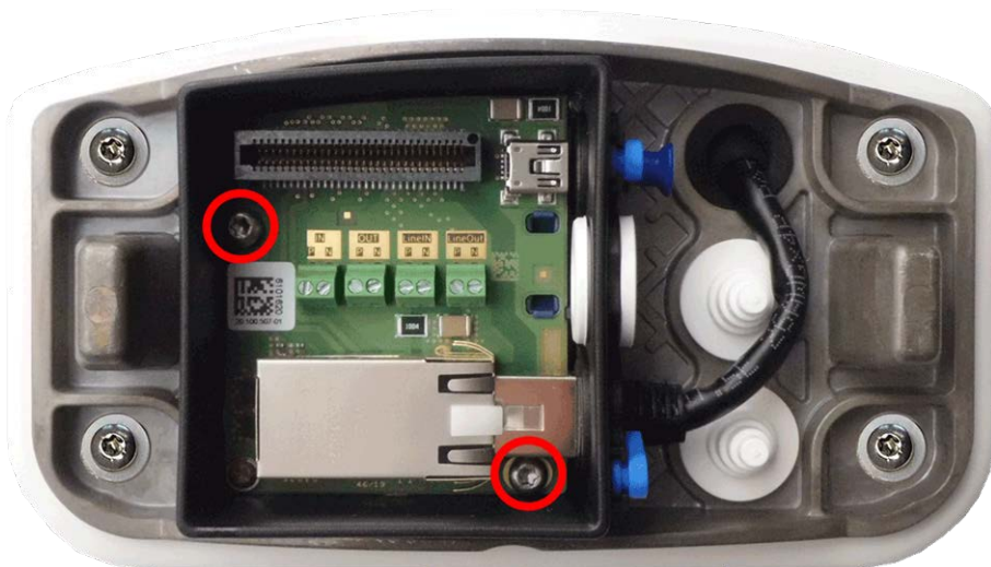
Fig. 55: Mount the Connector Box RJ45 (top view) using the two screws (highlighted red in the figure) on the mounting plate
