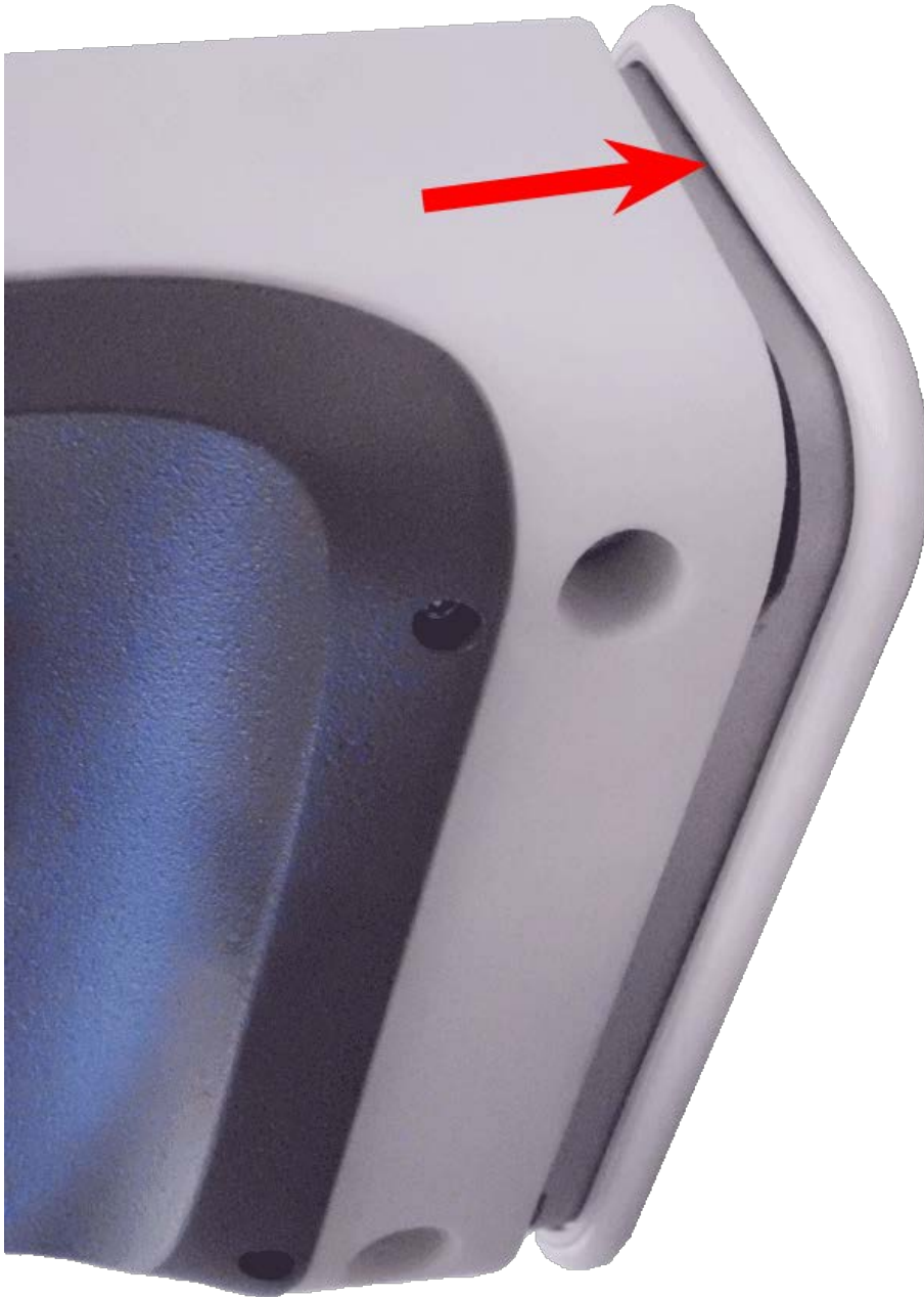
Fig. 69: Press camera onto mounting plate
