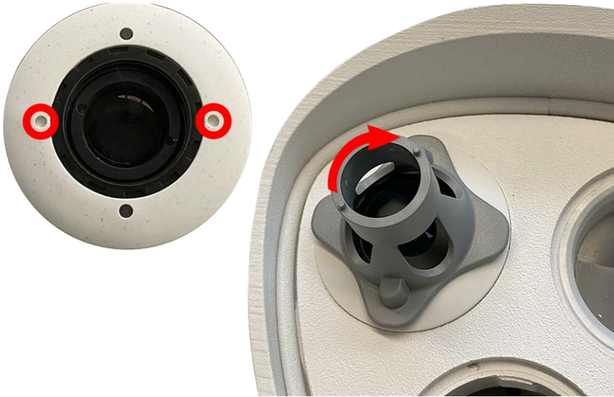
Fig. 13: Lock the sensor module
