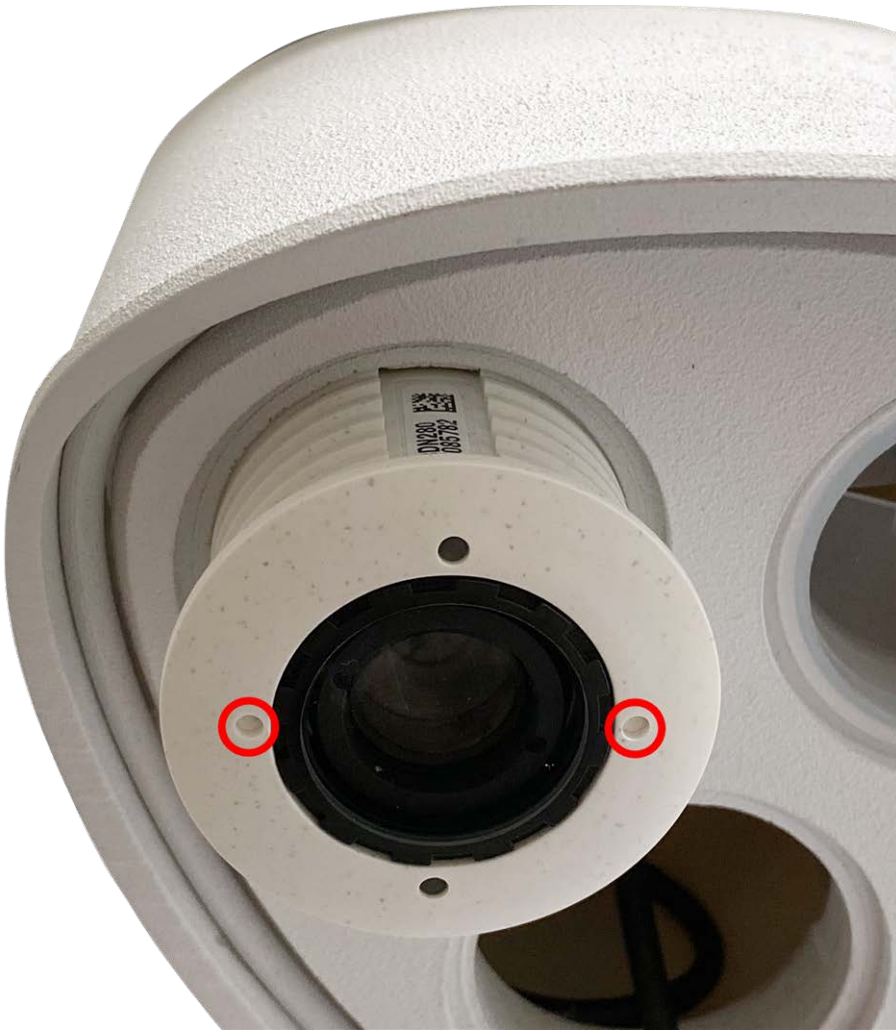
Fig. 12: Insert sensor module into module housing
