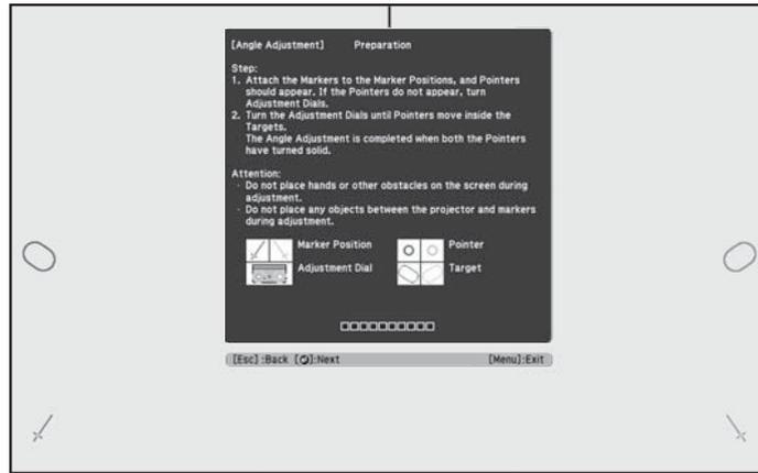
11. Turn the adjustment dials on the Touch Unit to move the circles ○ so that they move inside of the target (○) (○) of the same color (blue and green) on either side.
