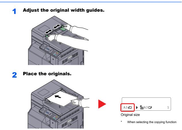
Put the side to be scanned (or the first side of two-sided originals) face-up. Slide the leading edge into the document processor as far as it will go.
