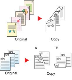
Produces two-sided copies from one-sided originals. In case of an odd number of originals, the back side of the last copy will be blank. The optional duplex unit is required.
