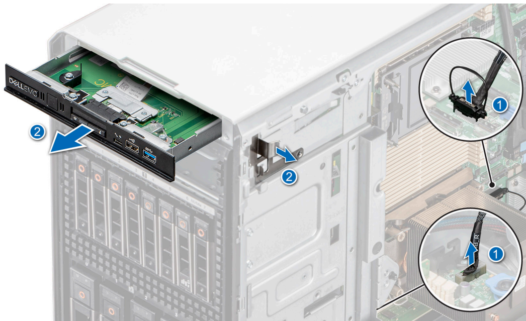
Figure 102. Removing the front IO module for upsell configuration
