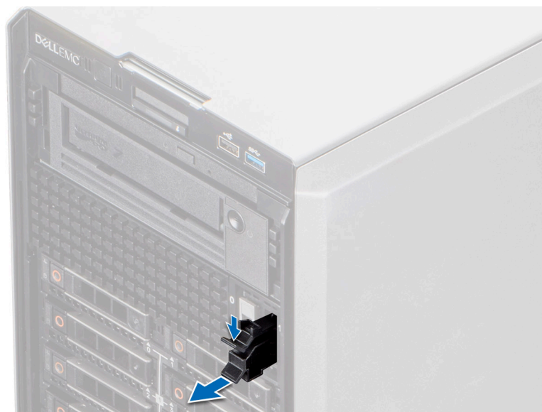
Figure 117. Removing the BOSS S2 card carrier blank
