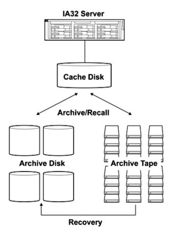
All archived data is initially cached on Cache Disk for rapid access and immediately committed to the archive layer for long-term retention. The combination of online access and large capacity MSA1500 with the LTO WORM tape library provides a level of media longevity and record authenticity that cannot be matched by a monolithic disk archive, positioning the Archive Solution as an optimal replacement for Magneto-Optical and UDO Jukeboxes.
