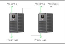
Live standby redundancy
