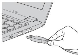
The first time you plug a USB device into a particular USB port on your computer, Windows automatically installs a driver for that device. After the driver has been installed, you can disconnect and reconnect the device without performing any additional steps.
