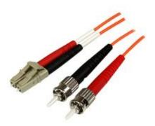
The 50FIBPLCST1 1m LC to ST Plenum Fiber Cable features 50/125 micron fiber for high-speed, high bandwidth data transmissions over Gigabit Ethernet and Fiber Channel networks, with support for duplex multimode applications.
