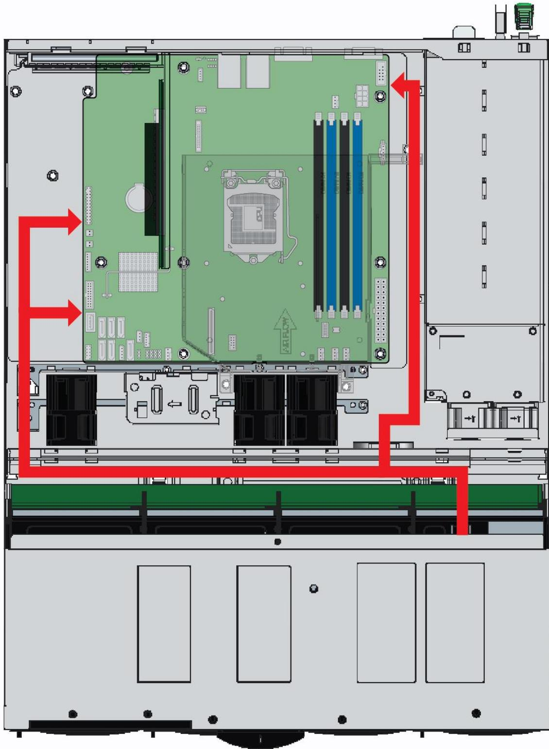
Figure 48. Internal Cable Routing
