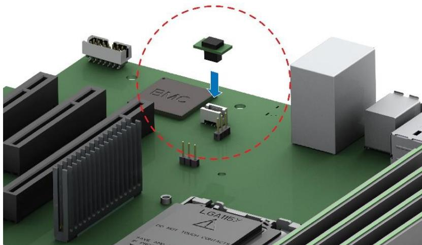
**Figure 46. Intel® RMM4 Lite Activation Key Installation**
