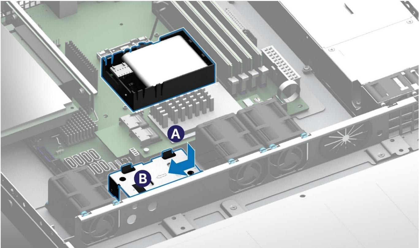
Figure 40. Intel® RAID Maintenance Free Backup Unit
