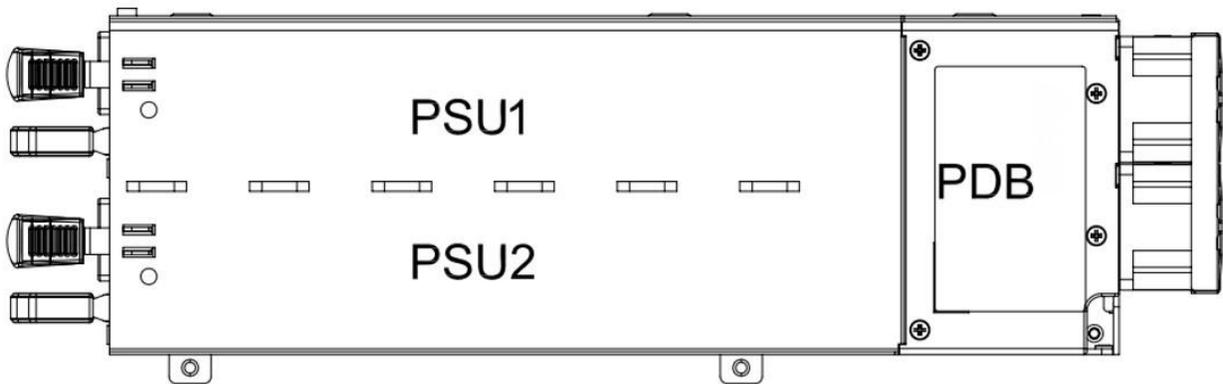
Figure 22. Power Distribution Board
