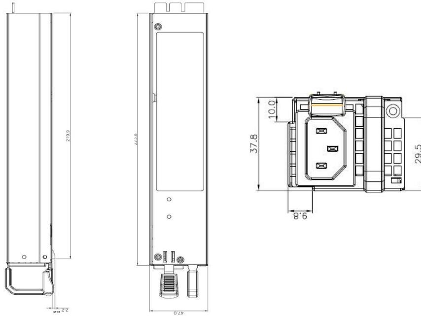
Figure 21. 450W Power Supply Mechanical drawings
