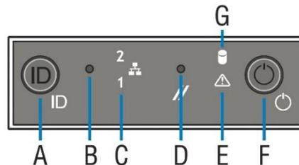
**Figure 42. Front Panel LEDs and Buttons**
