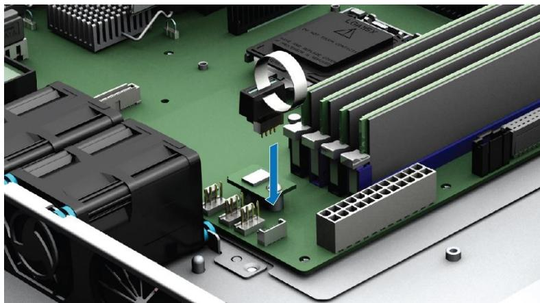
Figure 39. Intel® Raid Upgrade Key
