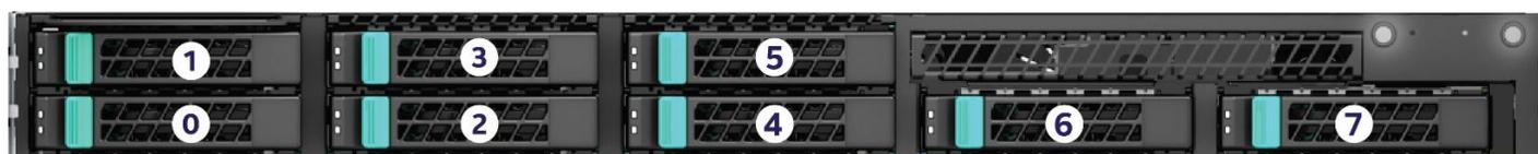
Figure 28. 8x2.5" Drive Bay Configuration (Model R1208xxxxx)
