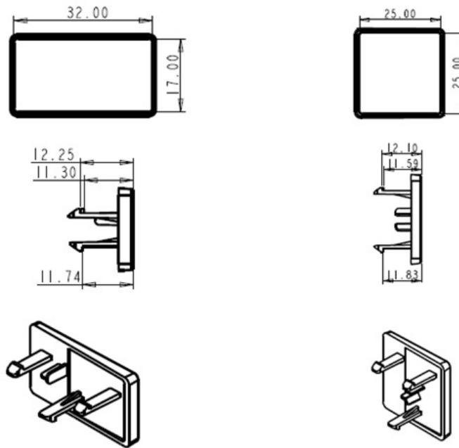
Figure 14. Front Bezel Accessory ID Badge Mechanical Drawings
