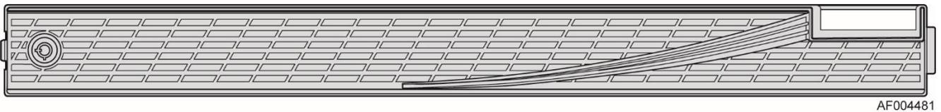
**Figure 11. Front Bezel Accessory with Optionally Installed Wave Feature**
