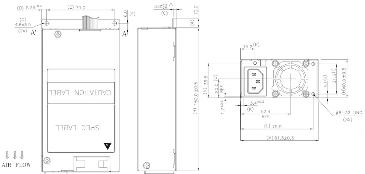
**Figure 20. 350W Power Supply Mechanical Drawings**
