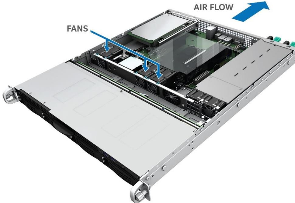
**Figure 24. System Air Flow and Fan Identification**
