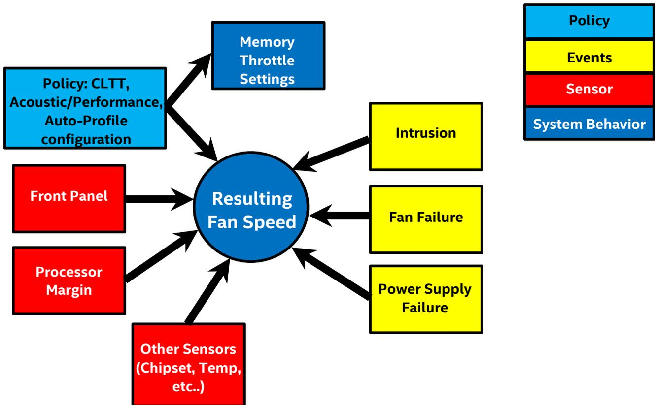
Figure 25. Fan Control Model
