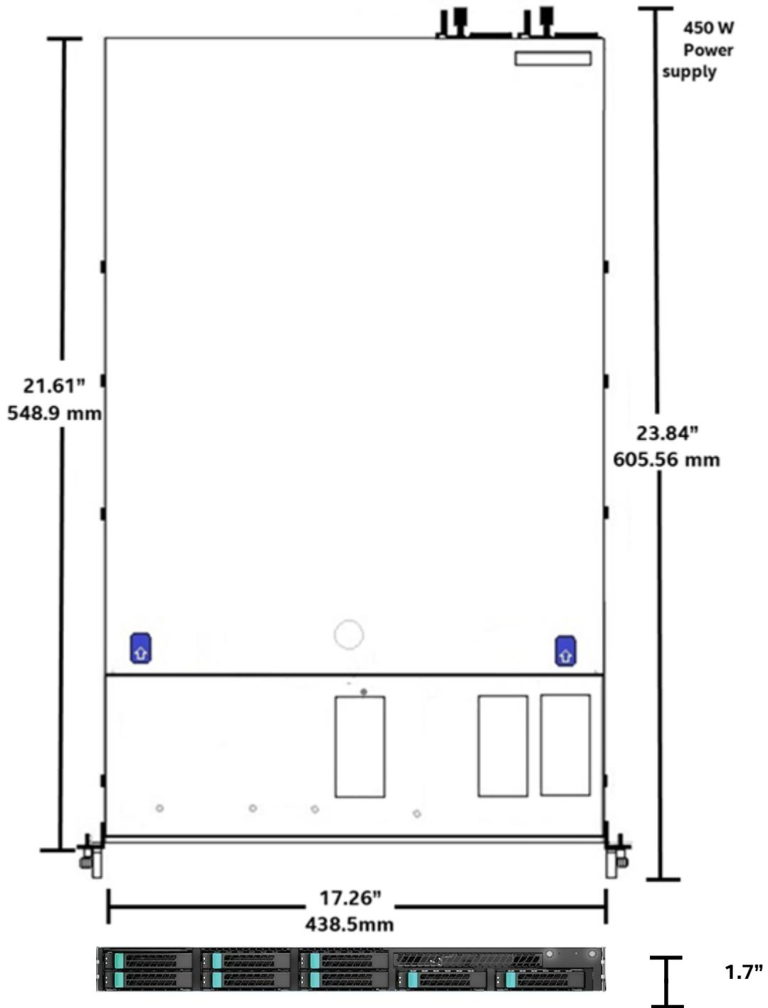
Figure 15. Chassis Dimensions
