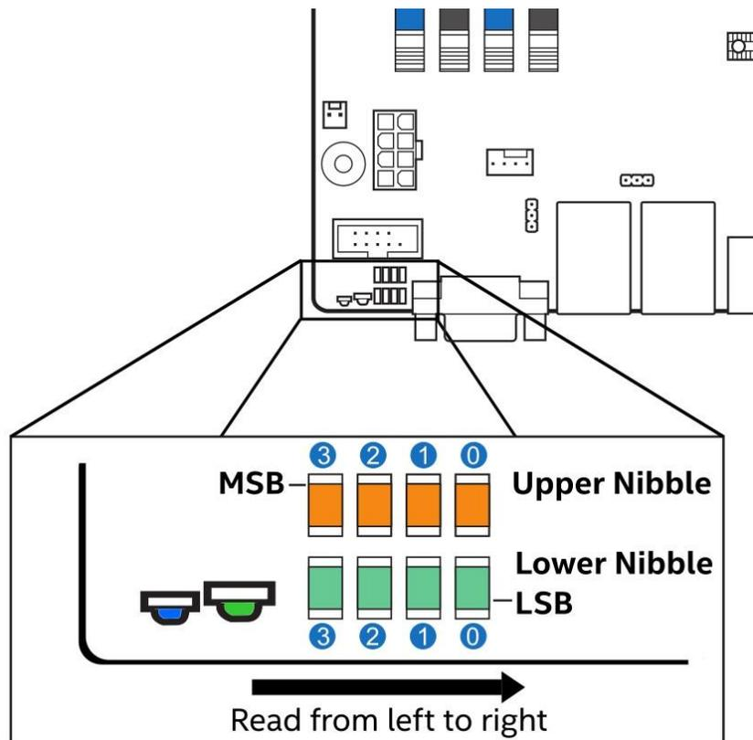
**Figure 47. POST Diagnostic LED Location**
