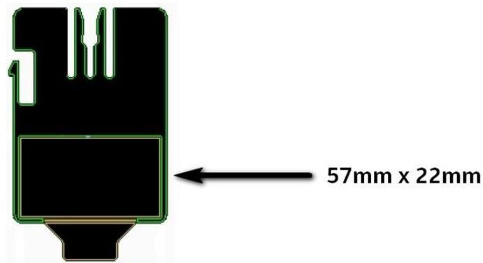
Figure 17. Pull-out Tab Label Emboss Dimensions
