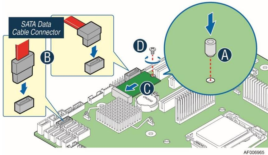
**Figure 38. Installing M.2 Device**
