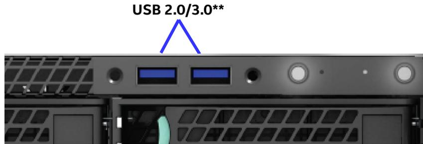
**Figure 41. Front I/O Panel Features**
