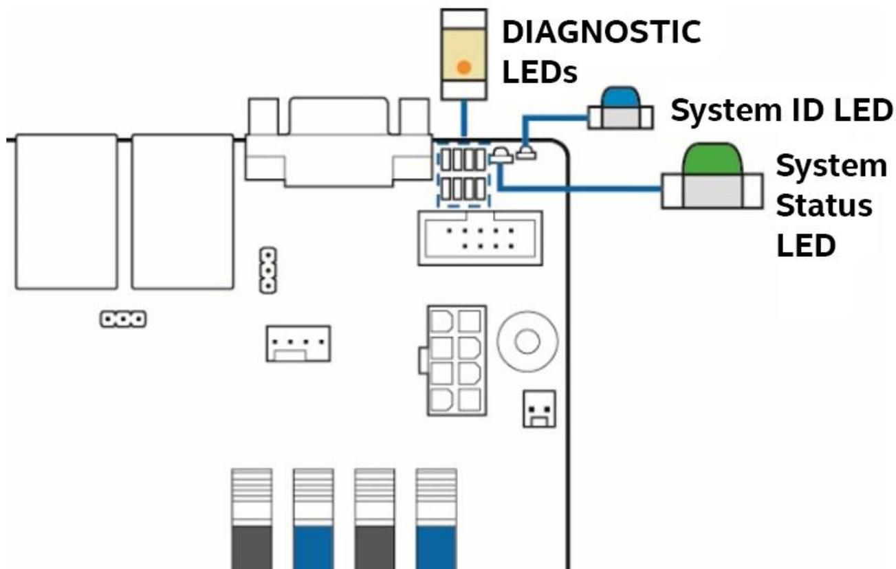
Figure 4. On-board Diagnostic LEDs
