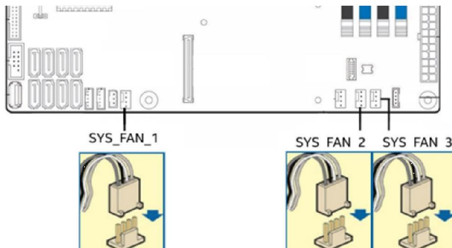
Figure 27. System Fan Connector Locations on Server Board
