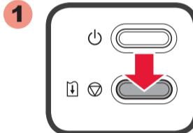
If the **Alarm** lamp flashes orange, press the **RESUME/CANCEL** button, then proceed to next chapter. Print Head Alignment can also be performed after installation.
