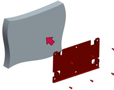
Mount the wall bracket to the wall using 6 fasteners appropriate for the type of wall structure following all applicable building code standards.
