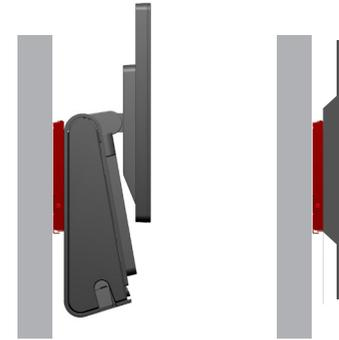
Hang the AiO on the wall bracket and secure using 2 M3 screws included with the kit on the left and right side of the bracket.
