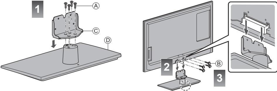
Secure the base as shown to prevent the TV from falling over.
