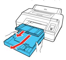
2. Remove any jammed paper from the front of the printer.
