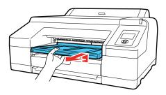
2. Move the lock lever to the unlock position.
