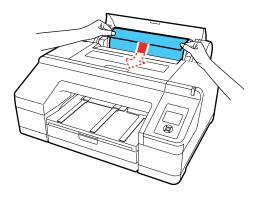
8. Press the \*\( \) load paper button on the control panel. The printer automatically feeds the paper to the printing position.
