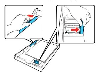
10. Insert the paper cassette and push it firmly into the printer.
