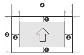
**Note:** Margins may change depending on the Roll Paper Margin setting that you select. The numbers below are the default settings. When printing with the left and right borderless setting, the left and right margins are 0. When printing with the borderless on all sides setting, all margins are 0.
