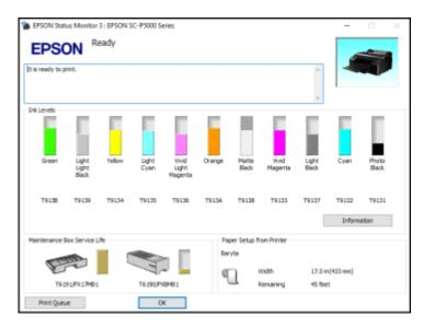
2. Replace or reinstall the maintenance tank or ink cartridge as indicated on the screen.
