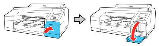
2. Use the handle on the bottom of the maintenance tank to carefully pull it out of the product without tilting the tank.
