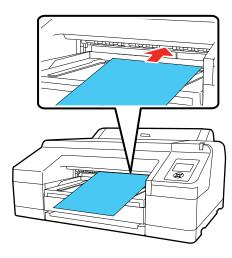
6. Look through the printer window and make sure the paper is inserted under the gray roller inside the printer.
