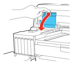
6. Loosen the screw holding the cutter in place and carefully remove the cutter.
