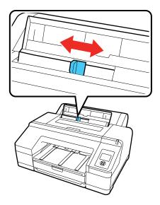
6. Insert a single cut sheet into the rear manual feeder, printable side up, until it reaches the gray rollers inside the printer.
