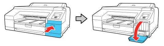
3. Press in on the ink cartridge you want to replace. The ink cartridge pops out slightly.
