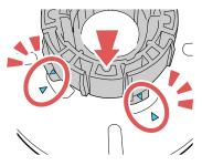
3. Insert the other gray adapter onto the spindle and attach it to the other paper stop.
