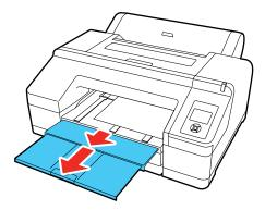
10. When printing is finished, press the \(^{\frac{1}{3}}\), load paper button to release the pressure roller so you can pull out the paper.
