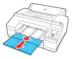
**Note:** If you are printing on plain paper or thin media types, or if you are using the optional Spectroproofer, raise the paper eject support. This prevents paper from curling up in the output tray, which can cause paper jams and print head strikes.
