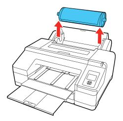
4. Remove the jammed paper from the roll paper feeder and/or the front manual feeder.
