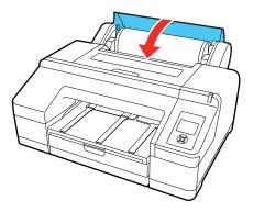
**Note:** To prevent dust from accumulating inside the printer, always keep the roll paper cover closed unless you are loading or unloading media.
