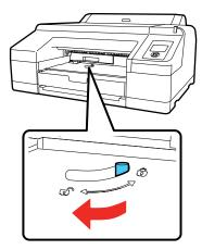
3. Use the handle on the bottom of the maintenance tank to carefully pull it out of the product without tilting the tank.
