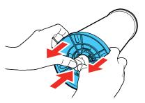
5. Remove the roll paper from the spindle.
