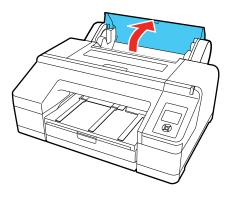
6. Remove the protective film from the cleaning sheet.
