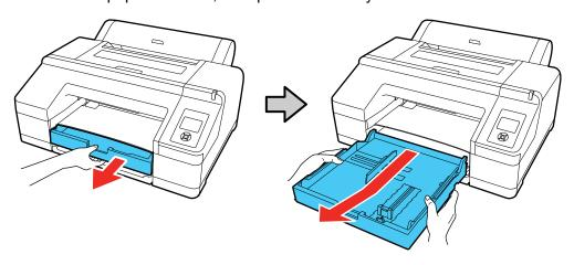
**Note:** If you are loading paper that is  $13 \times 19$  inches ( $330 \times 483$  mm) or larger, pull the lever in the paper cassette to extend it as far as possible and expand the slider all the way to the edge of the paper cassette.
