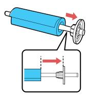
5. Insert the black paper stop onto the spindle and press in until there is no gap between the paper stop and the roll paper.
