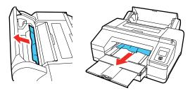
5. Open the printer cover and remove any other jammed paper as necessary.
