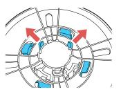
3. To remove the gray adapter from the other paper stop, slide it off the spindle.
