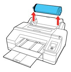
4. Remove the black paper stop from the spindle as shown.
