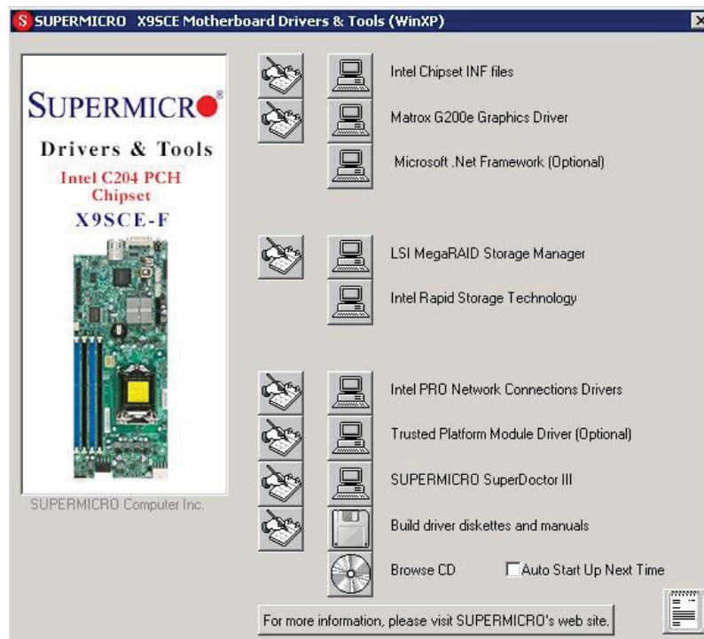
Figure 5-6. Driver/Tool Installation Display Screen
