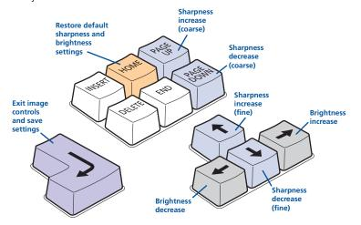
Sharpness: 1 U for fine adjustment, E for coarse adjustment.
