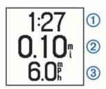
Time ①, distance ②, speed ③, total ascent, and calories are recorded while the timer is running. When using an optional heart rate monitor, your beats per minute and heart rate zone appear.
