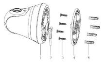
With the included screws and anchors, fasten the mounting bracket onto the wall. Before mounting the camera, the camera should be plugged into the AC adapter. Then, reattach the base cover and screw the stand back onto the mounting bracket.
