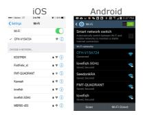
Before connecting to the camera, please turn on the Wi-Fi on your device as well as your personal Wi-Fi network. Then, go to your device Settings → under the Wi-Fi settings, connect to the CFH-V15XXXX (last 4 digits of the MAC ID, as seen on the back of the camera) network. Make sure that you see the Wi-Fi symbol after connecting to the camera.
