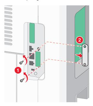
4 Insert the fax card and attach the two provided screws to secure the fax card mounting bracket.
