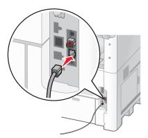
**3** Connect the other end of the telephone cord into the N slot of an active telephone wall jack.
