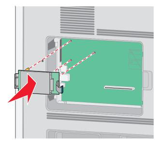
**b** Attach the two provided screws to secure the printer hard disk mounting bracket.
