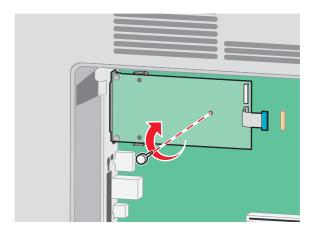
Attach the two provided screws to secure the ISP mounting bracket to the system board cage.
