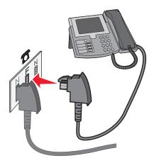
**5** If you would like to use the same line for recording messages on your answering machine, connect a second telephone line (not provided) between the answering machine and the other N slot of the telephone wall jack.
