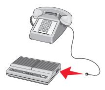
**5** Connect a third telephone cord from the answering machine to the EXT port of the printer.
