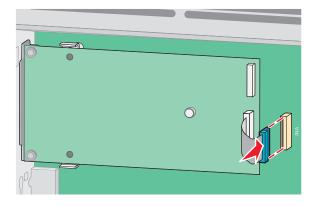
If a printer hard disk was previously installed, then attach the printer hard disk to the ISP. For more information, see "Installing a printer hard disk" on page 38.
