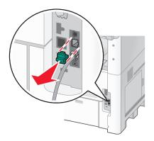
**2** Connect your telecommunications equipment directly to the EXT port on the back of the printer.
